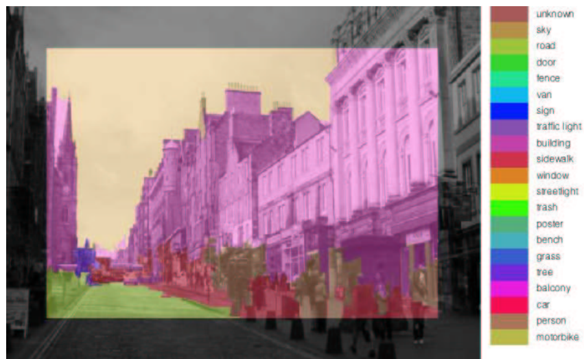
Figure 2: Street scene parsing: a convolutional network was trained on the LabelMe spanish dataset [8] with a method similar to [5]. The training set only contains photos from spanish cities; the image above is a picture taken in Edinburgh. The convolutional network is fully computed on neuFlow , achieving a speedup of about 100x (500x380 images are processed in 80ms, as opposed to 8s on a laptop).
